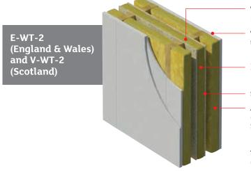
**Wall width:** 240mm (min) between inner faces of wall linings. 50mm (min) gap between wall panels
