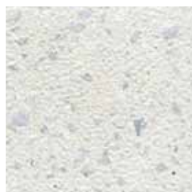
sandblasted surface with white aggregate
