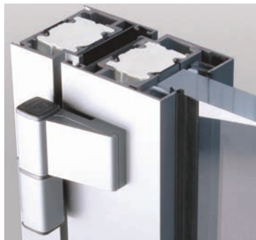
The fire protection core, which is anored in the middle, leaves space free on each side, which can be used for cable routing or for fastening add-on parts.
