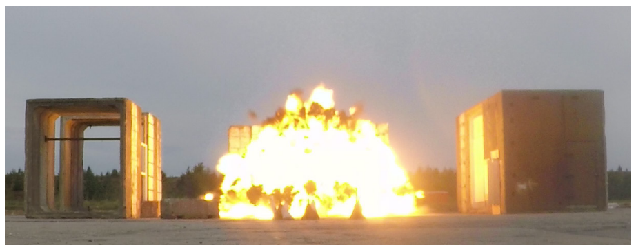
StoVentec Glass before and after blast testing
