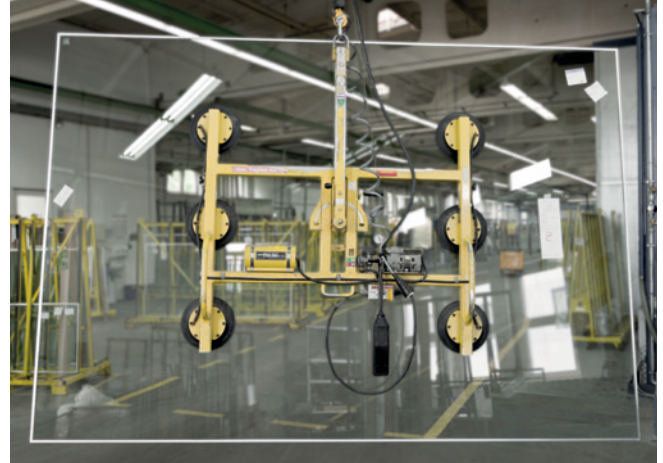
Vacuum suction cups must be evenly distributed across the surface of the glass pane.
