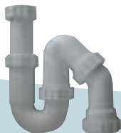
S2373001 - Tubular All in One Trap 75mm Seal Adjustable to Provide 'S' 'P' or 'Q' Type Connection. Adjustable inlet-32mm White Plastic S2373011 - Tubular All in One Trap 75mm Seal Adjustable to Provide 'S' 'P' or 'Q' Type Connection. Adjustable inlet-38mm White Plastic S2373021 - Tubular All in One Trap 75mm Seal Adjustable to Provide 'S' 'P' or 'Q' Type Connection. Adjustable inlet-50mm White Plastic
