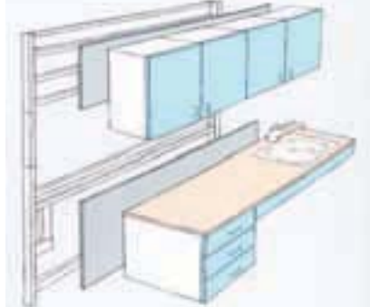
Worktop, base and wall unit adjustment
