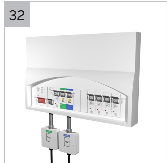
32 Isolate main supply and connect each pump to a separate non-switched fused spur. When installing a Delta HLA, follow the wiring diagram in Section 6.
