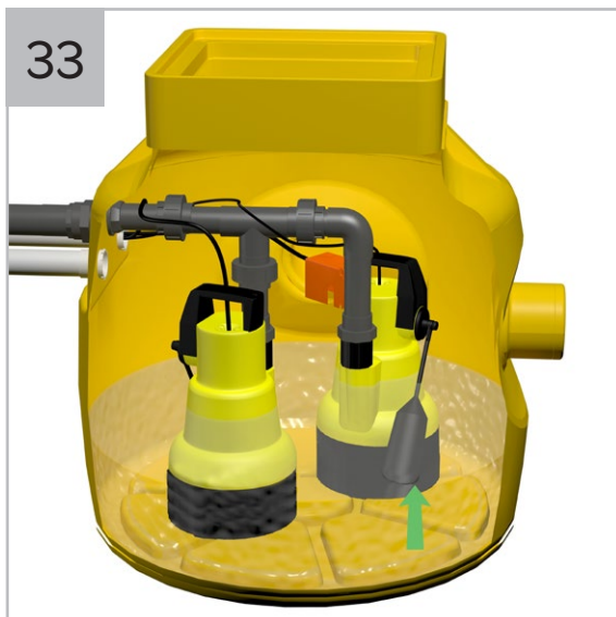
33 Ensure finger float is correctly installed vertically in shroud and not caught on float arm. Turn mains supply on and lift each pump float arm to test water is discharging correctly.
