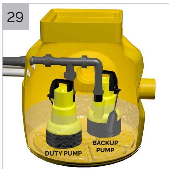
Lower the pumps in to chamber. Ensure 'O' rings are correctly seated in unions and screw discharge arms into place. The duty pump (low float arm setting) should be closest to the discharge. The backup pump (high float arm setting) should be at the rear so that its float arm cannot be obstructed by the float cable.
