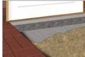
Step 3. Haunch around channel with concrete or suitable fill material.
