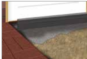
Step 2. Lay 50mm (min.) bed of concrete or mortar. Position the channel and fit to Ø110mm pipework, use a suitable adaptor coupling.
