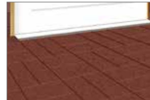
Step 4. Complete the installation by sealing between the door sill and grating.
