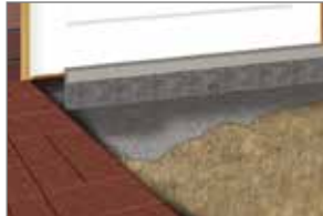
Step 2. Lay 50mm (min.) bed of concrete or mortar. Position the channel and fit to U-PVC Ø40mm pipework.
