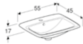
Geberit Selnova Square 55cm countertop basin W 55 / D 45 / H 17cm Visible overflow.
